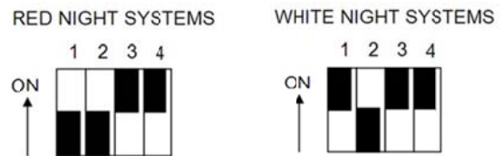
Figure 2-4 – PCB2 Micro/Filter SW1 Configuration
