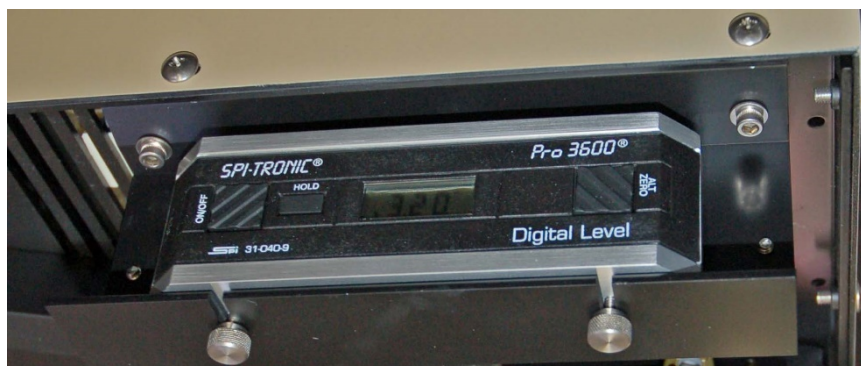
Inclinometer inserted in mounting bracket on the bottom of the LHA
