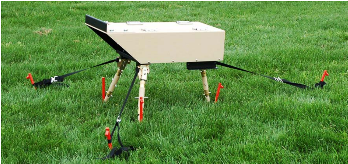
Fully secured LHA with ground stakes and straps
