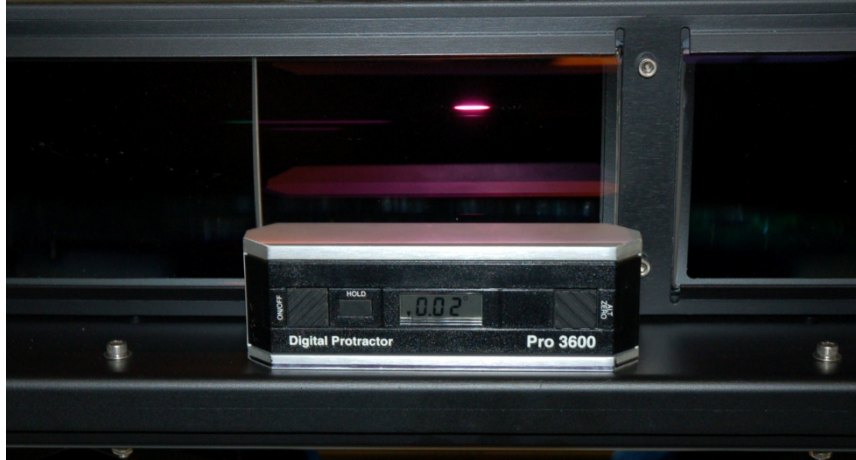
LHA with the digital inclinometer in place
